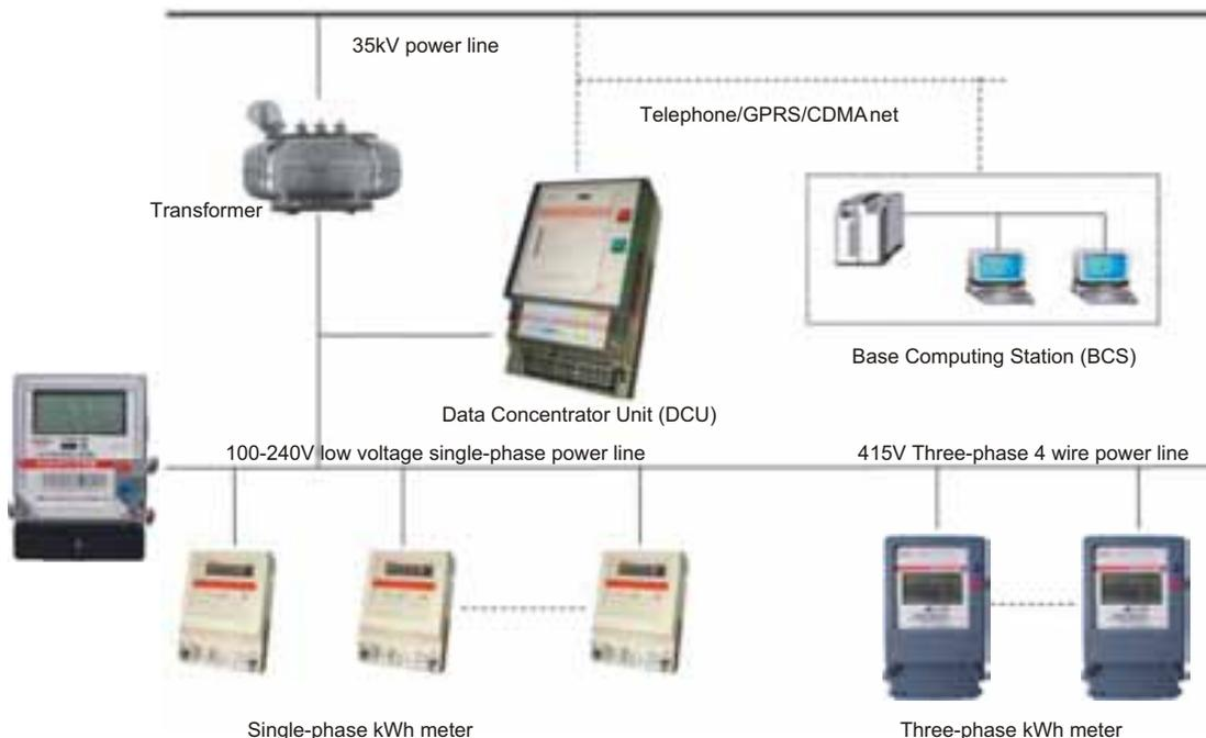
Figure 1 - A Sample Application of AMR System
